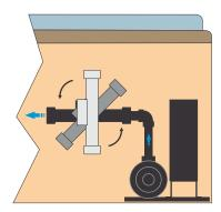
The heater can be installed vertical, horizontal or at an angle in the pumps discharge plumbing (providing position DOES NOT allow air pockets to form inside the housing). The heater can be installed up to 5-feet from the control system, which is connected via a black 3-conductor and black 6-conductor cord to the black receptacles provided at the control box..
