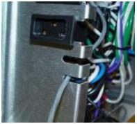
Route the flow switch cable through an empty slot allocated for small cables/cords.
