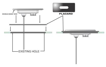
Step 1 - (If control cutout already exists, determine if placard must be used. If existing cutout is sufficient, disregard step 1.) Choose a location for the spaside control. Using the template provided, drill two 1" diameter holes, 2 5/8" apart. Cut away the material between the two holes, clean area and insert spaside. (If placard is required, position and secure using a water resistant silicone sealant.)
