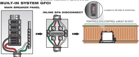
Power from main breaker panel to service disconnect within line-of-site of the spa to portable spa control equipped with buit-in GFCI.
