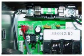
Connect the flow switch connector to the connection point making sure all pins are covered.
