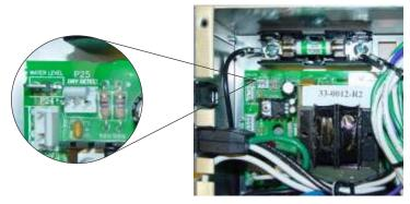
1. Locate the connection point for the flow switch.
