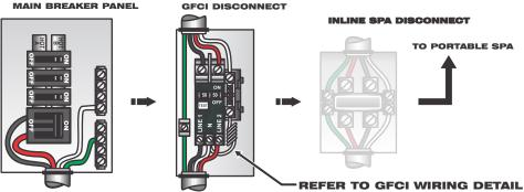
Power from main service panel to a GFCI subpanel within line-of-site of the spa. (Note: Most local codes will allow a GFCI subpanel to be a disconnect. If this is not the case in your installation, a disconnect must be provided.)
