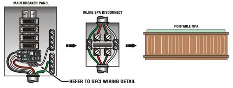
Power from GFCI breaker installed into main service panel to a service disconnect within line-of-site of the spa.
