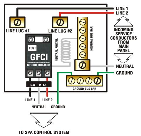
LOAD NEUTRAL <u>MUST</u> BE CONNECTED DIRECTLY TO GFCI AS SHOWN
