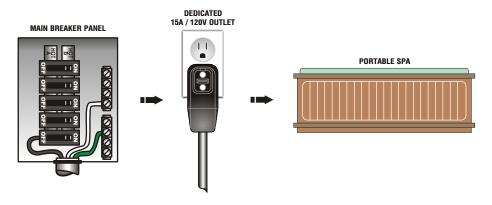
This illustration depicts a typical 15 AMP, cord-end GFCI installation. (The spa must be installed on a dedicated circuit.)
