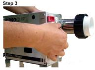
The mounting studs are attached to adjustable clamps on the heater. Loosen the clamps to adjust the stud locations to align with the slide brackets on one end. Do not tighten the nuts yet.
