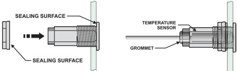
**Option #2 Heater Housing:** The "VS" / "US" Series heaters comes with 1/4" sensors located under the plate. To install the sensor, loosen the wing nut and slide the sensor under the plate until it becomes no longer visible. Once the sensor is install under the plate, tighten the wing nut to ensure the sensor is secure. If you wish, you can order the 10' x 3/8" temperature sensor to replace the existing temperature sensor for "Drywell" applications.
