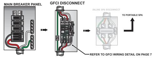
Option 2 shows the power from main service panel to a GFCI subpanel within line-of-site of the spa. (Note: Most local codes will allow a GFCI subpanel to be a disconnect. If this is not the case in your installation, a disconnect must be provided.)
