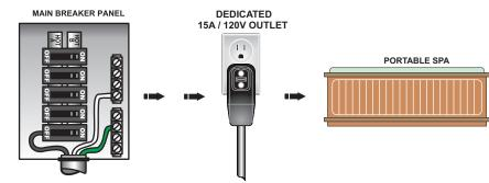
This illustration depicts a typical 15 AMP, cord-end GFCI installation. (The spa must be installed on a dedicated circuit.)
