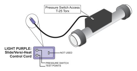
IMPORTANT: After any pressure switch adjustment, it is important to test the control by turning on the pump low speed and heater. While operating, unplug the pump, the heater must turn off. If the heater stays on, plug the pump back in and readjust the pressure switch to achieve proper operation.
