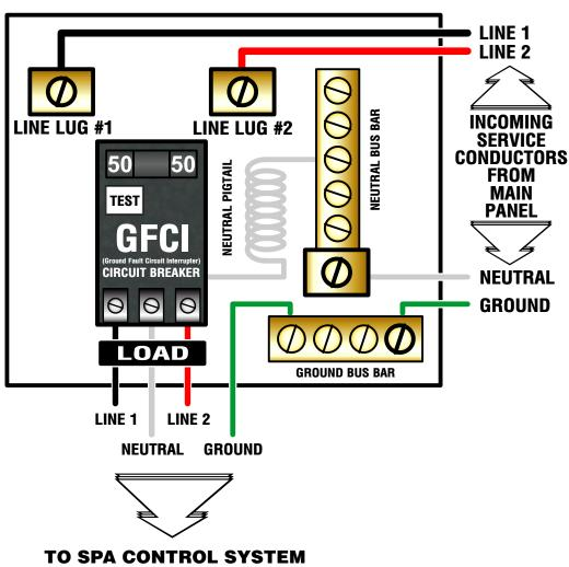
LOAD NEUTRAL MUST BE CONNECTED DIRECTLY TO GFCI AS SHOWN
