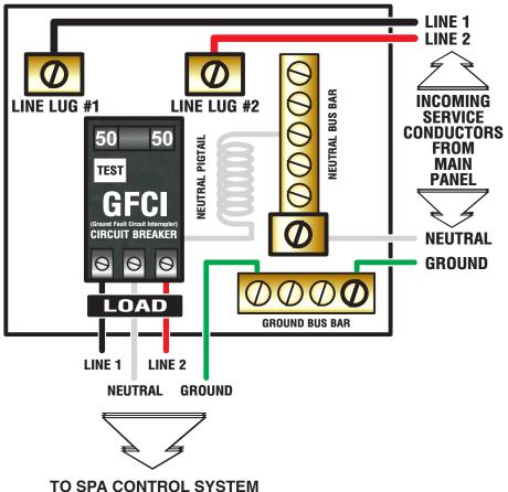
LOAD NEUTRAL MUST BE CONNECTED DIRECTLY TO GFCI AS SHOWN
