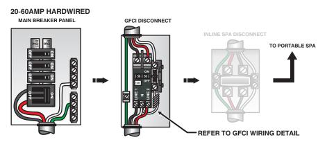
Power from main service panel to a GFCI subpanel within line-of-site of the spa. (Note: Most local codes will allow a GFCI subpanel to be a disconnect. If this is not the case in your installation, a disconnect must be provided.)
