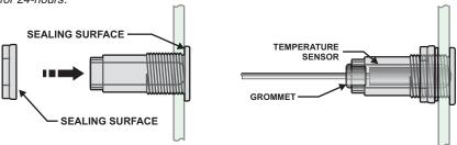
**Option #2 Alternate Method - HEATER HOUSING:** If it is not possible or desired to drill a hole into the spa shell the temperature sensor may be installed with the High-Limit sensor directly on to the heater housing under the sensor shield/cover. Simply loosen, insert probe as shown and re-tighten.
