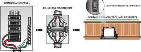
Power from main breaker panel to service disconnect within line-of-site of the spa to portable spa control equipped with buit-in GFCI.
