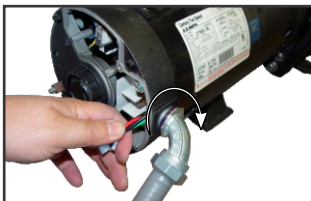
4) While holding the wires as shown thread the liquid-tight connector into the pump until secure then connect the power wires to the pump per the label on the pump.
